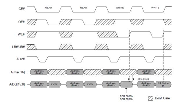
Figure 14: Read Configuration Register
