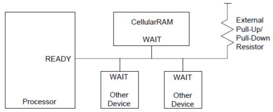
When a burst READ or WRITE operation has been initiated, WAIT goes active to indicate that the Cellular RAM device requires additional time before data can be transferred. For burst READ operations, WAIT will remain active until valid data is output from the device. For burst WRITE operations, WAIT will indicate to the memory controller when data will be accepted into the Cellular RAM device. When WAIT transitions to an inactive state, the data burst will progress on successive clock edges.
