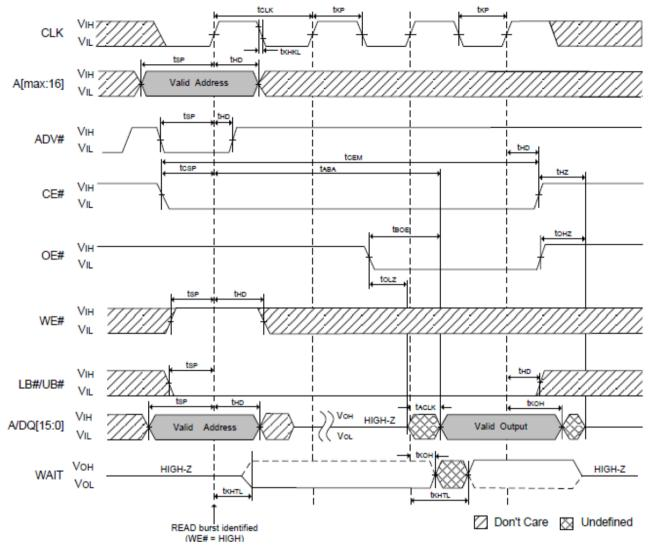
Note: Non-default BCR settings: Latency code two (three clocks); WAIT active LOW; WAIT asserted during delay.
