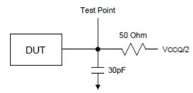
Note: All tests are performed with the outputs configured for default setting of half drive strength (BCR [5:4] = 01b).
